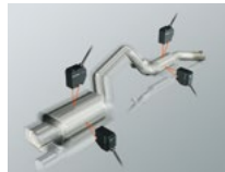
Vibration test of high-temperature-muffler
