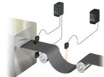
Thickness measurement/loop control of a rubber sheet
